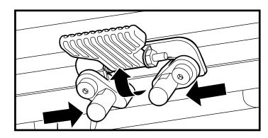
Figure 12. Seat Height Adjustment - Seat Latch Safety
